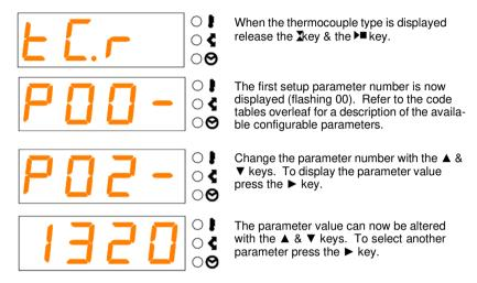
Pressing both the Xkey & the ▶■ key at any time causes the configuration parameters to be stored. The instrument will then reboot.
