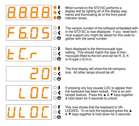
If any mimic panel lamps are on then the ST215C is firing. To stop the firing press the ▶■ kev.
