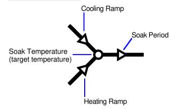
An ST215C firing segment comprises a ramp followed by a soak period. Two segments can be used for simple firing (biscuit firing for example) or several segments can be used per program for complex firing (crystal glazing or glass-making for example).
